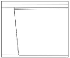
**INCORRECT!** Door is out of alignment with the rest of the unit.
