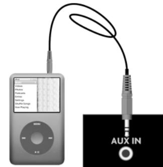
**TIP** (NOTE: This input is not muted when in the guitar tuner is in use).
