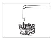
② The tightness of the tremolo arm can be adjusted by the torque adjustment cap. Turning the cap clockwise will make the arm tighter, and turning it counterclockwise will make the arm looser.
