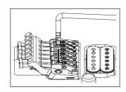
② The tightness of the tremolo arm attachment can be adjusted by adding or removing Teflon washers. Using a larger number of washers will make the attachment tighter, and removing all the washers will leave the arm free. The Teflon washers can be added or removed diagonally via the slit.
