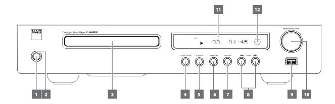
1 STANDBY BUTTON: Press this button to switch ON the C 546BEE. The Standby LED indicator will turn from amber to blue and illuminate the Vacuum Fluorescent Display (VFD). Pressing the Standby button again turns the unit back to standby mode.
