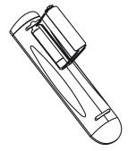
Replace battery cover by aligning and inserting the two tabs into the holes. Press battery cover into place until it "clicks" closed.
