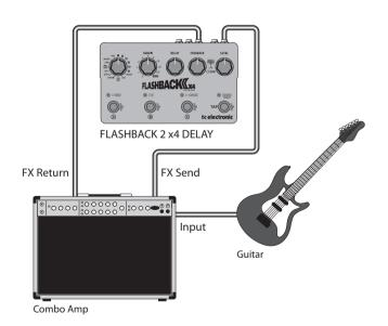
The FLASHBACK 2 X4 input can handle a very wide range of signal levels thanks to high internal headroom, and can easily be used with guitar or line-level signals. Simply connect the amp's Send jack to the the pedal's input, and connect the output to the amp's Return jack.
