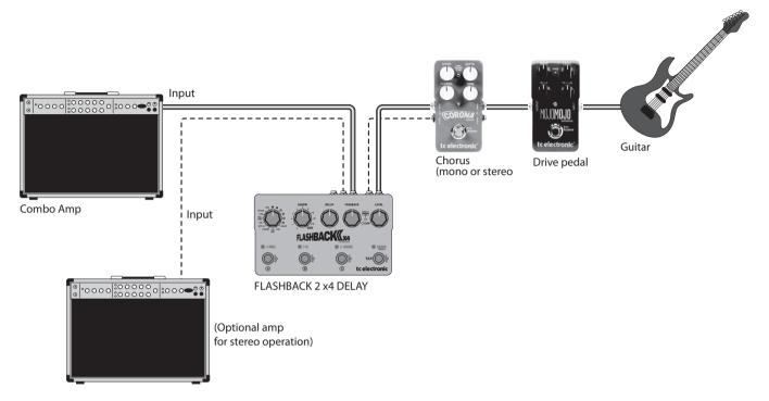
When using the FLASHBACK 2 X4 before the amp's input, it is generally best to place it after your other pedals. If any stereo effects are used before the delay pedal, you can preserve this stereo signal by connecting to both of the FLASHBACK 2 X4's inputs and sending the output jacks to different amps or to a stereo input on a mixer.
