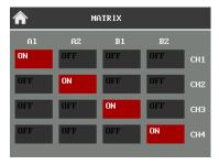
The Matrix page allow users to manage the routing of the four input channels to the four output channels.
