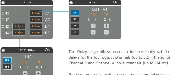
Pressing on a delay value, users can set the delay in ms or in mt. Press the OK button to return to the Delay page.
