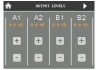
The Levels page allows users to independently manage the amplitude of all the four input channels and all the four output channels.
