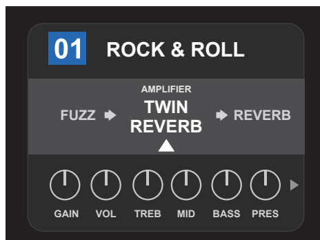
Flanked by two effects, the amp model within the preset is selected here in the SIGNAL PATH LAYER, as indicated by the white arrow and the word “amplifier.”
