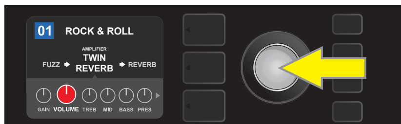
Press the ENCODER to select an amp model control knob for adjustment.
