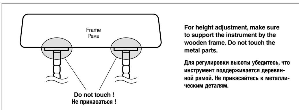
Lift the frame ends to the desired height and then securely tighten each slide leg fixing bolt, aligning it with the corresponding notch of the slide leg. Bolt and notch are aligned when the next higher notch is flush with the upper leg flange. (Refer to step 8 on page 29.)
