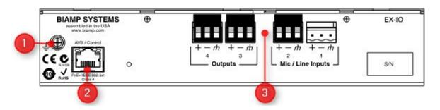
EX-IO expander pictured. The type and number of inputs and outputs will vary depending on expander model
