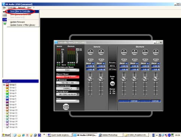
Fig. 28: FirNet™ – Opening the dialog box for loading individual filters
