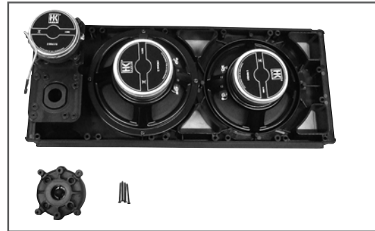
Fig. 37: Dismantled CAD 208 baffle board with the woofer
