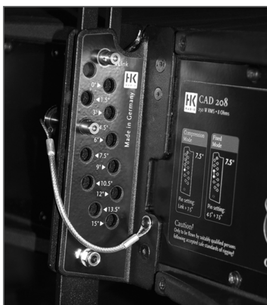
Fig. 12: The CAD 208's set angle in compression mode is 4.5°
