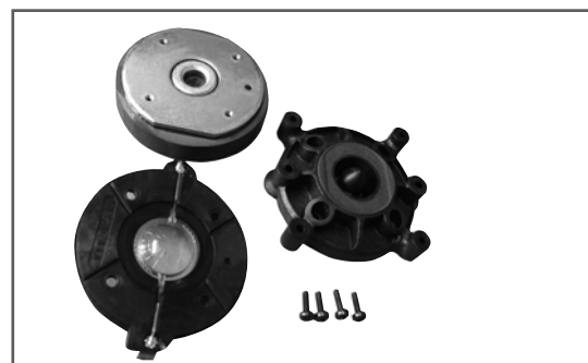
Fig. 38: Voice coil removed from the CAD 208 HF driver
