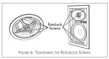
· When you notice resistance on the screws the speaker has been clamped successfully.
