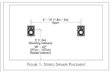
speakers can be placed at various ceiling heights while still providing good coverage for all listeners.
