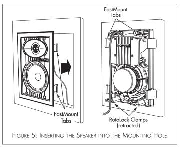
NOTE: The FastMount tabs are designed for one-time use only. If the speaker is removed from the mounting hole the FastMount tabs will disconnect and remain inside the wall or ceiling.
