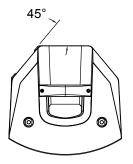
Note that only one angled back panel has footing ridges to stabilize the speaker when positioned as a floor monitor
