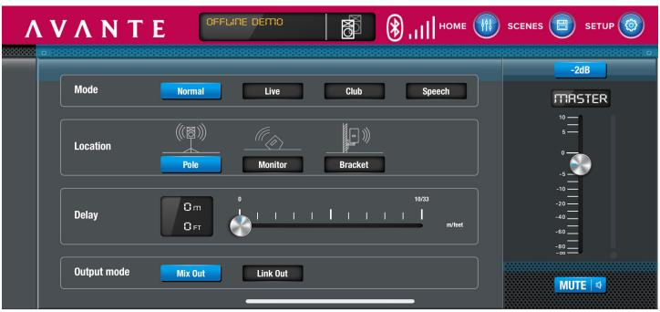
Master Channel Page: adjust the volume, mode, Location, delay, and output mode of 2 channels.
