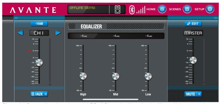
**Channel 1 Page**: adjust the volume and EQ of Channel 1. Note that the Master Volume can also can adjusted here.
