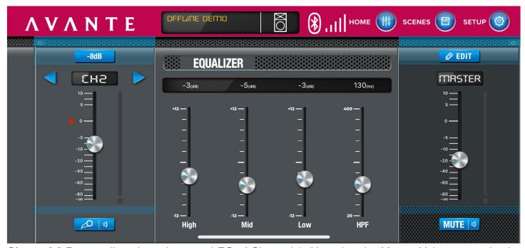
Channel 2 Page: adjust the volume and EQ of Channel 2. Note that the Master Volume can also be adjusted here.
