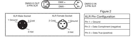
**Special Note:** Line Termination. When longer runs of cable are used, you may need to use a terminator on the last unit to avoid erratic behavior. A terminator is a 110-120 ohm 1/4 watt resistor which is connected between pins 2 and 3 of a male XLR connector (DATA + and DATA -). This unit is inserted in the female XLR connector of the last unit in your daisy chain to terminate the line. Using a cable terminator (ADJ part number Z-DMX/T) will decrease the possibilities of erratic
