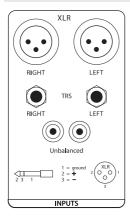
**Line-level Inputs:** The Temblor T10 provides a choice of three input pairs: two sets of balanced inputs (XLR and ¼"TRS) and one pair of RCA unbalanced inputs. When both of the balanced connections are in use, the TRS inputs will take precedence over the XLR inputs. The RCA inputs will sum into either balanced connection.
