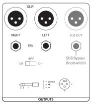
**Outputs:** The Temblor T10 provides two pairs of balanced outputs: XLR and ¼"TRS. The fullrange signal connected to the stereo inputs on the T10 is passed through to these outputs. Use these outputs to connect your main left and right studio monitors. If the High Pass Filter switch is engaged, frequencies below 80 Hz are not sent from these outputs.
