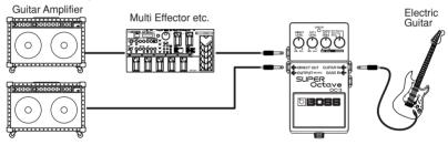
When the OC-3 is in DRIVE mode (p. 7) while DIRECT OUT is connected, the direct sound (without the distortion applied) is output from DIRECT OUT. Taking sounds with effects added using a multi-effects processor or other such device and the sounds in DRIVE mode and playing them through multiple amps allows you to produce an extremely low sound with greater separation. In such settings, the DIRECT LEVEL knob (p. 6) adjusts the direct sound level.
