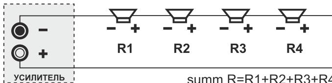
$$\text{summ } R = R_1 + R_2 + R_3 + R_4$$
