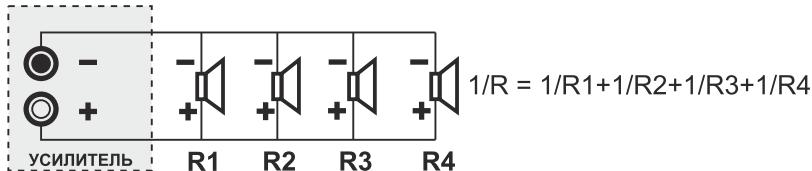
$$1/R = 1/R_1 + 1/R_2 + 1/R_3 + 1/R_4$$
