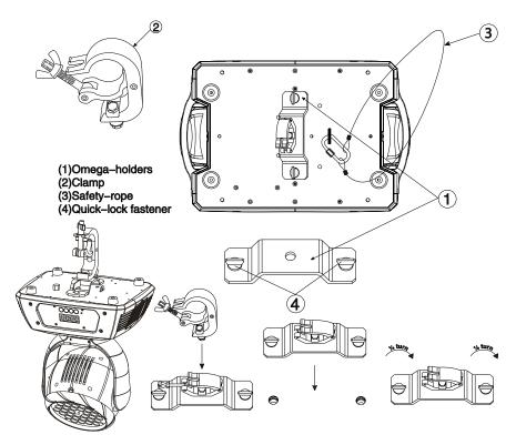
Screw one clamp each via a M12 screw and nut onto the Omega holders. Insert the quick-lock fasteners of the first Omega holder into the respective holes on the bottom of the Vizi Wash LED 108. Tighten the quick-lock fasteners fully clockwise. Install the second Omega holder. Pull the safety-cable through the holes on the bottom of the base and over the trussing system or a safe fixation spot. Insert the end in the carabine and tighten the safety screw.
