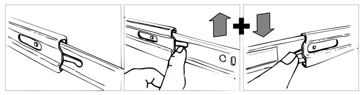
Fully extend drawer and locate plastic lever on drawer slide.
