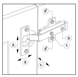
If the cabinet's doors appear out of alignment, this condition can be corrected with minor adjustment to the European hinges on each door.
