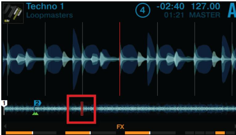
1. While holding **SHIFT**, place your finger on the Touch Strip beneath the orange LEDs and swipe to the right to move forwards in the track's waveform.
