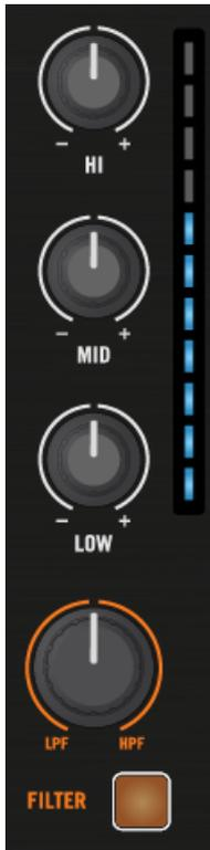
The EQ and FILTER knobs on channel B.
