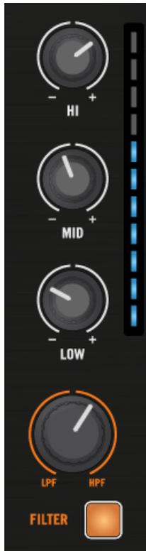
The EQs and filters are excellent tools for making adjustments to tracks before mixing them in so that you get the smoothest transition possible. The most common technique is to filter the bass line out of the incoming track—having 2 bass lines running simultaneously rarely sounds good.
