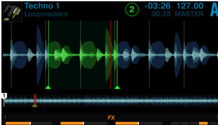
The step size you move the selection by is the same as the loop size, which is shown in the display.
