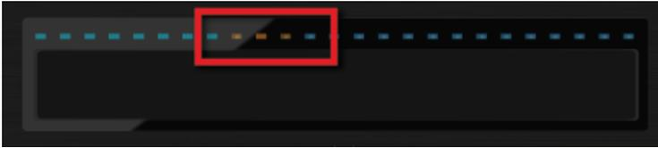
The LED segments represent the entire length of the track. The three orange segments represent the current playhead position within the track.
