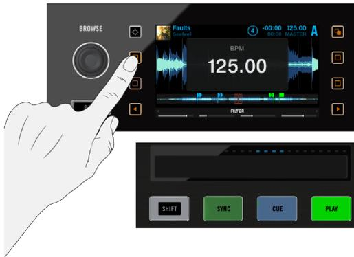
2. Turn the **BROWSE** knob to adjust **MASTER** tempo in .01 BPM increments. To adjust in full BPM steps, hold **SHIFT** while turning the knob.
