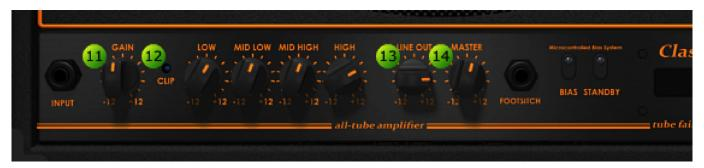
**13 Line Out** - The level of the sound of the head, but not the cabinet.
