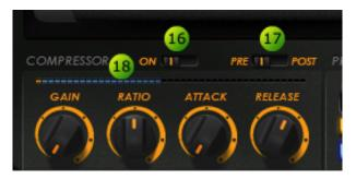
The **ratio** knob controls how much the compressor reduces the sound as the input rises: higher settings of this ratio will make loud passages more equal to soft passages.
