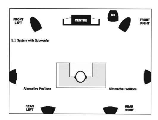
**Subwoofer:** As deep bass is fundamentally non-directional, this allows you to place a subwoofer in a variety of locations. Placing the subwoofer near a corner or particularly close to a wall will boost the bass but may impair clarity. Refer to your subwoofer manual for further information.
