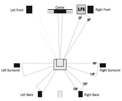
This is the recommended layout for 7.1 multichannel systems.
