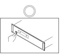
To avoid damage, please don't switch off the power until "no disc" or "time code" is showed on the LCD after the disc holder has been closed with the OPEN/CLOSE button.
