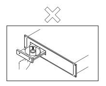
Do not switch off the power when the disc holder is open.
