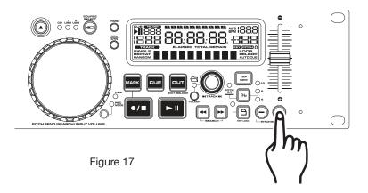
Holding down or tapping on the (+) *PITCH BEND BUTTON (12)* will provide a speed bump in the playback pitch.
