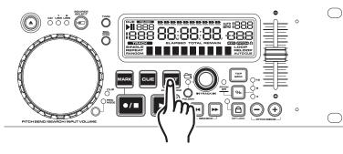
3) Press the OUT/EXIT/RELOOP BUTTON (18) to reactivate the SEAMLESS LOOP. Press the OUT/ EXIT/RELOOP BUTTON (18) to deactivate the loop.
