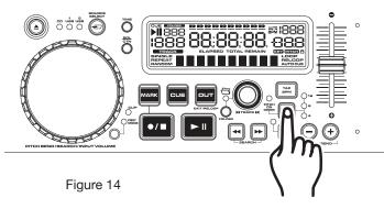
**Using the Pitch Slider (9):** To use the *PITCH SLIDER (9)* slide the slider up and down. Down will increase the pitch and up will decrease the pitch. When the slider is in the center position, there is zero pitch being applied to a track.
