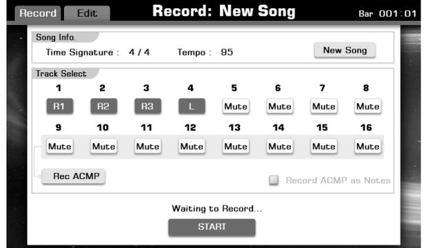
2. Play notes on the keyboard or press the [PLAY/ STOP] button to start recording. The [RECORD SONG] button will stop flashing and keep lighting.
