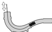
6. After removing all the water from the neck interior, dry with a cleaning swab drawn through the neck to remove all moisture.
