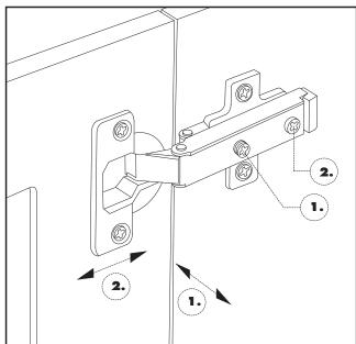
Use the **Phillips Screwdriver (A)** supplied to adjust Signal's door hinges:
