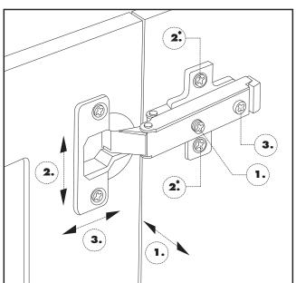
Use the **Phillips Screwdriver (A)** supplied to adjust Braden's door hinges:
