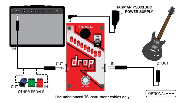
**NOTE:** The Drop should be the first pedal in your effects chain. Placing any effect in front of it can impact the pitch shifting performance.
