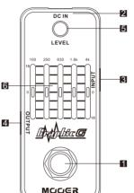
1. TRUE BYPASS Footswitch: Push down the footswitch to togale between on and bypass status.
