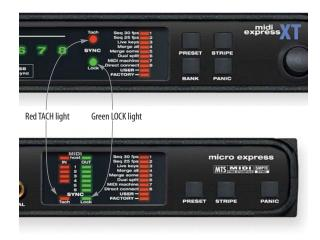
Figure 8-2: Converting time code. When your Express interface converts incoming time code, the red TACH light blinks, the green LOCK light glows steadily, and the green Computer I/O light glows steadily as well.
