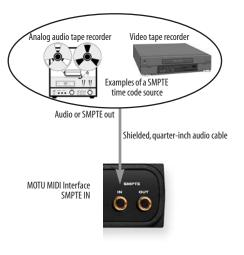
Figure 2-5: Connecting a SMPTE time code source.
