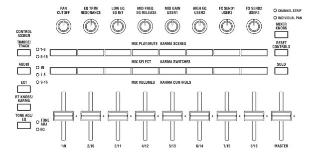
Use the MIX SELECT switches to select the input/track you want to control, and use the knobs to control them.
