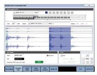
If you want to audition the selected region, press the Play button in the LCD or the SAMPLING START/STOP switch. The selected region will play at the pitch of the base key (the blue key in the keyboard display). You can specify the base key by holding down the ENTER switch and playing a note on the keyboard.
