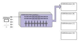
With the appropriate "ASSIGN" settings, a GE realtime parameter of (for example) module A can controlled independently by Master and Module A. For example you can make settings so that the Swing parameter of a drum GE on module A is controlled in MASTER by slider 1 over a range of 0-50%, and in MODULE A by slider 1 over a range of 50–100%.
