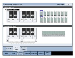
On the User Scale page, you can create your own original scales. These include sixteen different User Octave Scales, in which the pitch of each note of the octave is repeated for all octaves, and one User All Note Scale, in which the pitch of each of the 128 notes can be specified independently.
