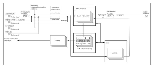
Each Sample is contained in an Index, which includes parameters for the key range, original Sample pitch, tuning, level, and so on.
