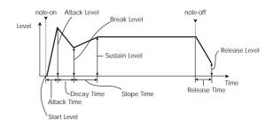
The HD-1 includes three EGs, for Pitch, Filter, and Amp. These produce time-varying changes in pitch, tone, and volume respectively. They can also be used to modulate a number of other Program parameters via AMS.
