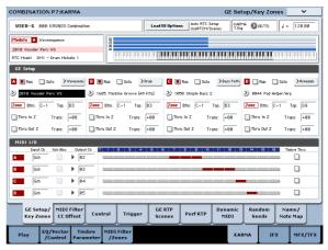
2. Use the "Run" and "Solo" settings to specify the module(s) that will operate when KARMA is on.
