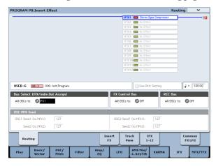
Use Bus Select (IFX/Indiv. Out Assign) to specify the bus to which the oscillator output will be sent. If you want the oscillator output to be input to insert effect 1, choose IFX1.
