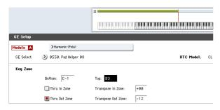
In the example shown above, the notes from C-1 through B3 are being input to the KARMA module. When you play B3 or a lower note, KARMA will generate a phrase or pattern.
