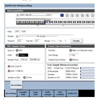
Under REC Sample Setup. note that **Sampling Mode** has been set to L–Mono. This means that the sound of the internal L channel will be sampled in mono.
