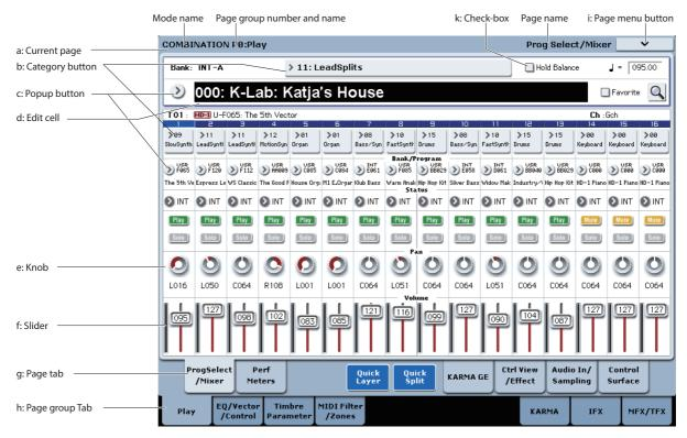
The KRONOS uses Korg's TouchView graphical user interface. By touching objects displayed in the LCD screen, you can select pages, set parameter values, move sliders and knobs, enter text, connect virtual patch cables, and more.
