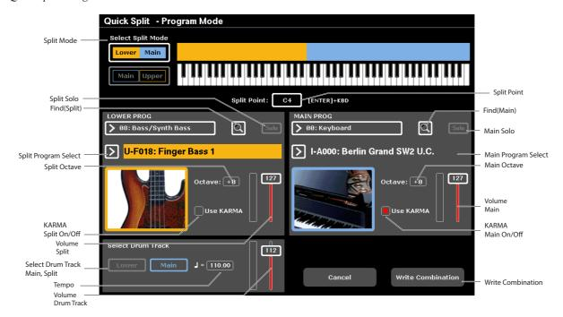
Quick Split makes it easy to create common setups, such as piano for the right hand and bass below for the left, or electric piano for the left hand and a lead synth for the right. Let's walk through the first example: a bass and piano split.
