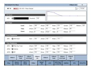
The Filter EG is a multi-stage envelope, which you can use to modulate the filter (naturally!) as well as other Program parameters. The EG itself is set up on the Filter EG tab; the way that it affects the filters is controlled by the parameters described below, on the Filter Mod tab:
