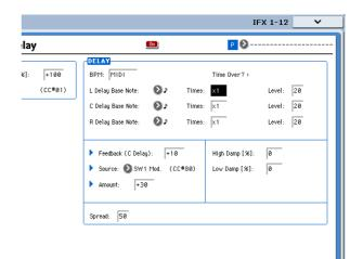
For this example, set **Delay Base Note** to and **Times** to x1 so that the effect will be easily understandable. The delay time will repeat at an interval of a 8th note.
