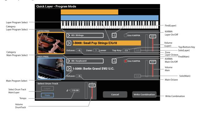
Here, we'll walk through a typical use of Quick Layer: adding a string layer to a piano sound. To do so:
