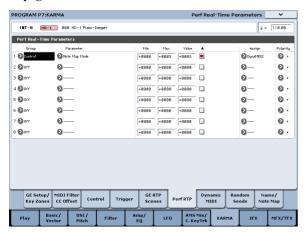
As an example, we'll show how you can use a KARMA CONTROLS slider to control the KARMA module parameter "Transpose."
