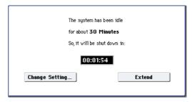
If you want to continue using the system, press the keyboard, a button, or some part of the display such as the Extend button. The Auto power-off function will be reset. If the specified length of time again elapses with no user input, the same message will appear again. You can also use the Change Setting button to bring up the Auto Power-Off Setting dialog, as described above.
