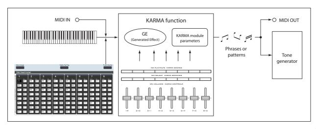
You can control the phrase or pattern by editing these parameters, or by assigning them to the KARMA CONTROLS sliders or KARMA SWITCH buttons and operating these during your performance.
