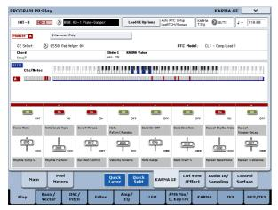
When you play the keyboard, the name of the chord detected by the KARMA module will appear in the "Chord" field of KARMA Module Info.
