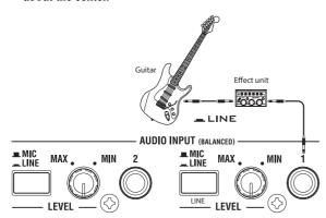
If you connect a guitar with passive pickups (i.e., a guitar that does not contain a preamp), you will be unable to sample it at the correct level because of the impedance mismatch. Such guitars should be routed through a preamp or an effect unit first, and then connected to the KRONOS.
