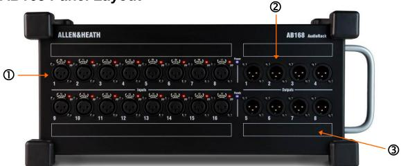
Input sockets 16 balanced XLR mic/line inputs with +48V Phantom Power indicator. The preamps are built into the AB168 and their Gain, Pad and 48V phantom power are remote controlled from the mixer via the dSNAKE link. The outputs of the analogue preamps are converted to digital format and transported via dSNAKE to be processed and mixed at the GLD or Qu mixer.
