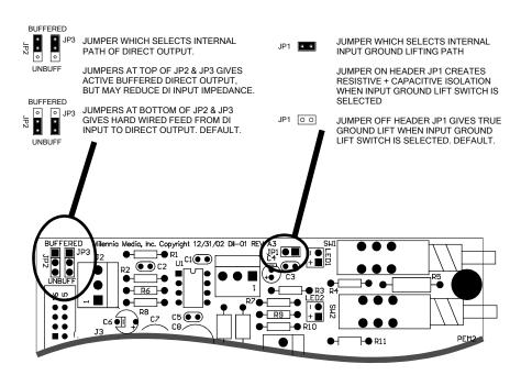
Direct Output Buffered / Non-Buffered Output Jumper Input Ground Lift / Isolate Jumper — Input Board
