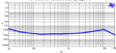
TD-1 Line / Mic THD (Active Balanced +27 dBu output)
