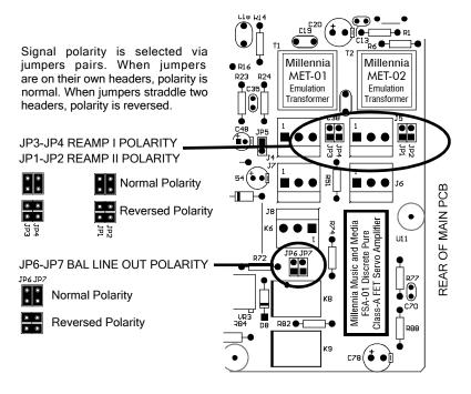
Reamp and Balanced Line Output Polarity Jumpers – Main Board
