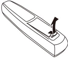
② Install new batteries into the compartment.
