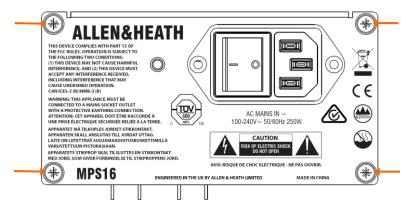
(i) dLive MixRacks ship with one PSU fitted. A second PSU can be fitted for redundancy (part number MPS-16). Loosen the 4 captive thumb screws securing the blank panel\*, slide the PSU into the slot, and tighten the 4 captive thumb screws indicated above. The MixRack will automatically switch between the supplies without interruption to the audio should one fail.
