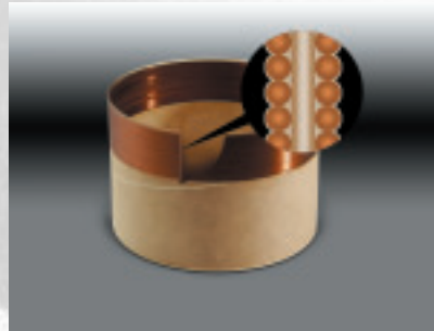
Voice coil wound 'Inside/Outside' for more effective cooling.
