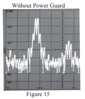
PG light and a dynamic electronic attenuator at the amplifier input reduces the input volume just enough to prevent any further increase in distortion. The Power Guard circuit acts so fast that there are absolutely no audible side effects and the sonic purity of the music reproduction is perfectly preserved. The MA6900 Amplifier with Power Guard is not limited to just the
