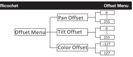
To enter the offset adjustment submenu, press the ENTER button for at least 5 seconds. In this submenu you are able to adjust the original position of the pan, tilt, gobo wheel, and color wheel.
