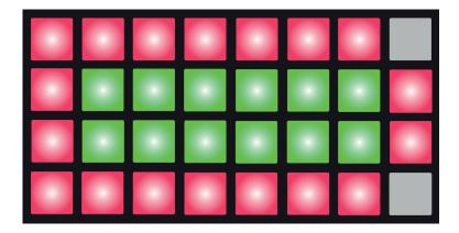
The diagram above shows the display when the batteries are fresh or at full capacity. The number of pairs of green pads give an idea of the battery condition; fewer green pads means the batteries are running down. When no green pads are showing, the batteries should be changed; otherwise you may lose your work.
