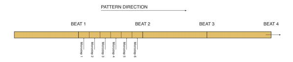
However you are not limited to merely shifting the timing – you can have a drum hit on as many microsteps as you want: each microstep pad is "on" or "off". Using *Drum Microstep View* can therefore add a whole new range of rhythmic possibilities to any pattern, and can create subtle yet quite funky rhythmic effects, As with many other aspects of Circuit, we urge you to experiment!
