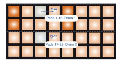
You can now add a snare drum to the sequence by pressing pads on the lower two rows. If you press **Drum 3** (or **Drum 4**), the sequence view for the other two drum tracks will be displayed, and you will find that you can add two other drum sounds at any step or steps in the sequence.
