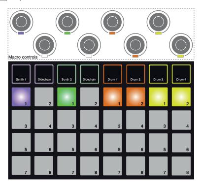
The six illuminated pads are effectively Mute buttons for each track. Press a pad to mute the track; the pad's illumination dims. Pressing a Mute button stops the sequencer triggering notes in the synth.
