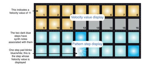
In *Velocity View*, the two lower rows of the grid represent the pattern steps. In the 16-step example shown above, Steps 4, 12 and 16 are brightly lit, indicating that these steps have notes associated with them. One pad in the Pattern step display will flash alternate white/blue: this is the step whose Velocity value is being displayed.
