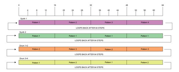
The above example illustrates the basic points involved in chaining Patterns together to make a longer sequence. Creating longer, more complex and more interesting sequences is merely an extension of these principles. Circuit allows sequences of up to 128 steps, with each of the four tracks changing pattern every 16 steps.
