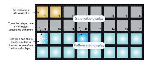
In *Gate View*, the two lower rows of the grid represent the pattern steps. In the 16-step example shown above, Steps 1 and 4 are brightly lit, indicating that these steps have notes associated with them. One pad in the Pattern step display will flash alternate white/blue: this is the step whose Gate value is being displayed.
