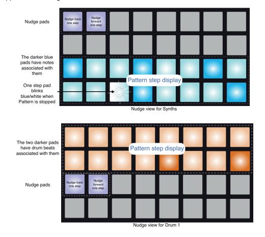
In either case, two pads are lit dimly blue; the left pad retards the selected pattern by one step each time it is pressed, the right pad advances it. The Nudge pads light white as they are pressed.
