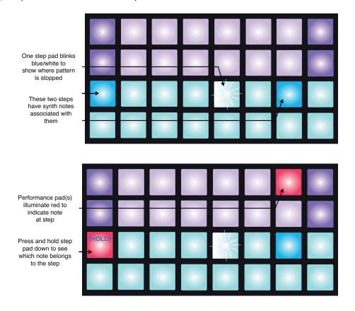
If a bright blue step pad (i.e., one corresponding to a synth note) is pressed and held, it illuminates red, the note(s) at that step will sound, and the performance pad corresponding to the note(s) will also illuminate red (it will be two pads if it's the highest note in the lower octave or vice versa). This is illustrated in the second diagram above. The pads stay red and the note(s) sound(s) for as long as the step pad is held down.
