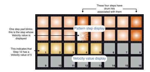
In *Velocity View*, the two upper rows of the grid represent the 16-step pattern for Drum 1 or Drum 3, while the two upper rows make up a 16-segment "bargraph" meter; the number of pads illuminated "sand" (off white) represent the Velocity value for the selected step. If Drum 2 or Drum 4 is selected, the pairs of rows are reversed, with the velocity meter above the steps.
