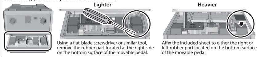
Using a flat-blade screwdriver or similar tool, remove the rubber part located at the right side of the bottom surface of the movable pedal.
