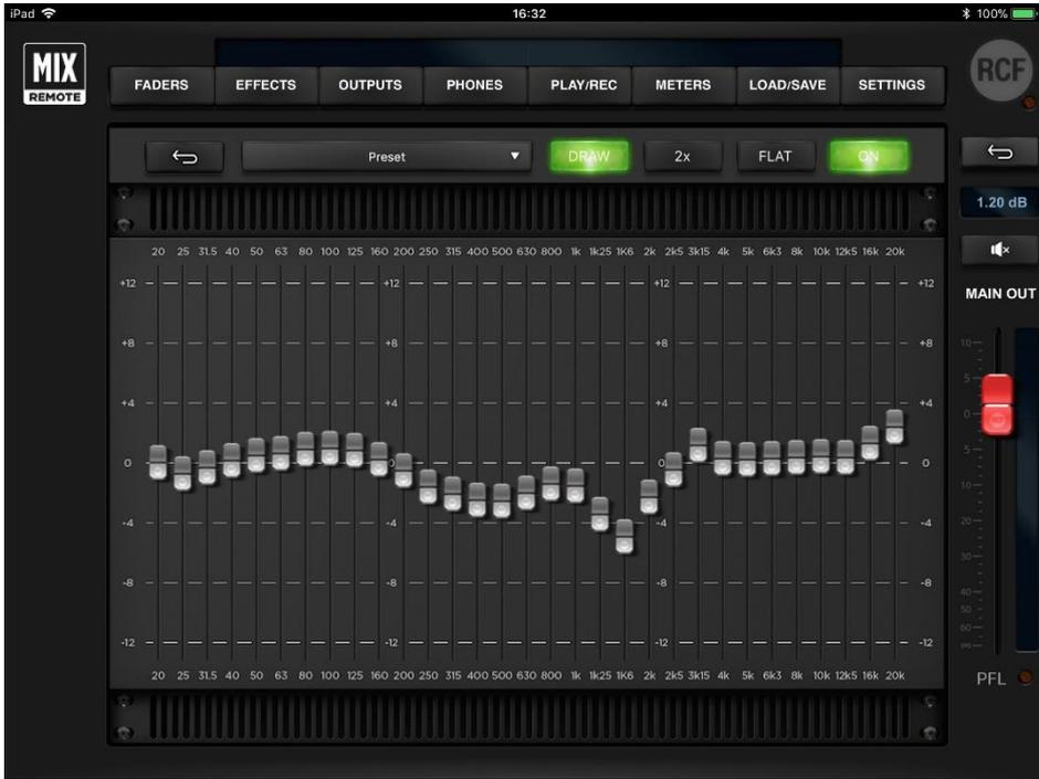
On the upper side there are: **Preset** dropdown to save and recall your custom settings, **DRAW** button that allow to manually design your equalizer curve, **2x** button to double the size of bands for a more accurate editing, **FLAT** button to set all bands to 0 dB and **ON** button to enable or disable the GEQ.
