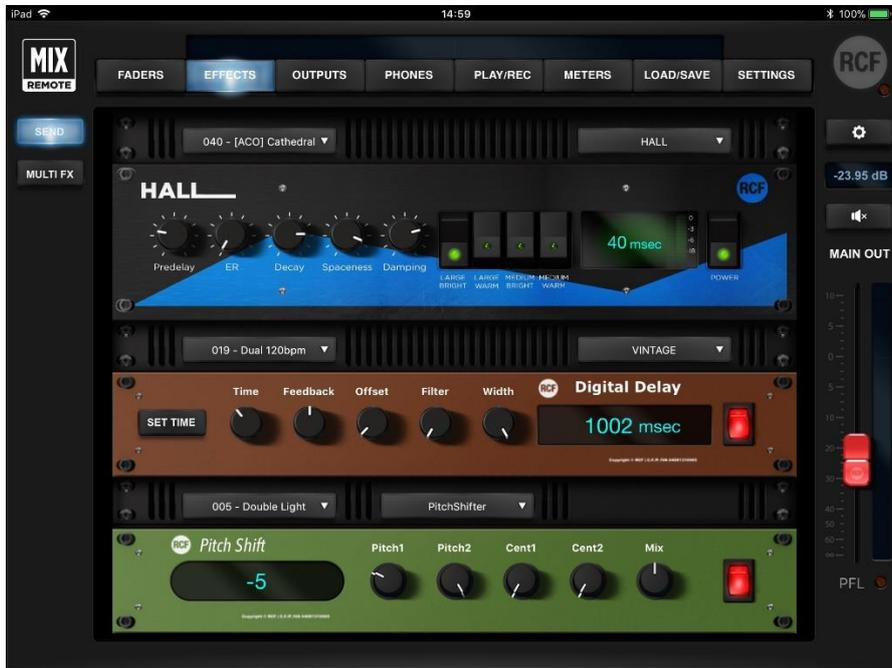
The left column shows the SEND and the MULTIFX select buttons; the right column shows usual the MAIN OUT controls.
