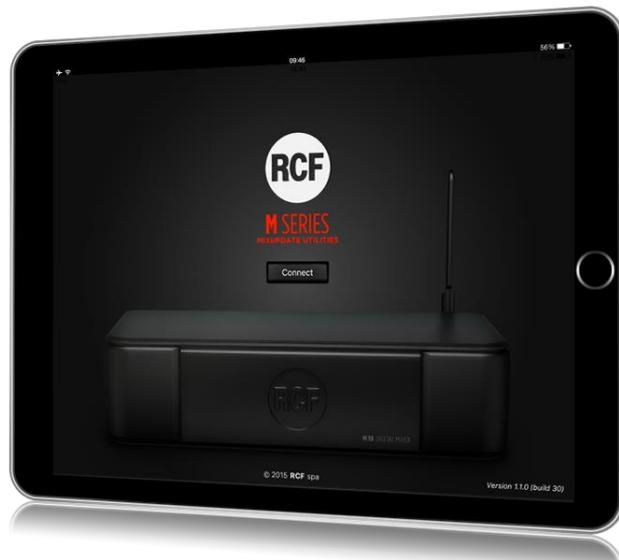
MixUpdate is a dedicated application for M 18 firmware update. MixUpdate for iOS also features BACKUP and RESTORE functions. BACKUP allows saving all the Snapshots, Shows and Effects' Patches from the mixer into a USB stick inserted in the M 18. Then, the RESTORE command brings the contents back to the M 18, either the same unit or a different one.
