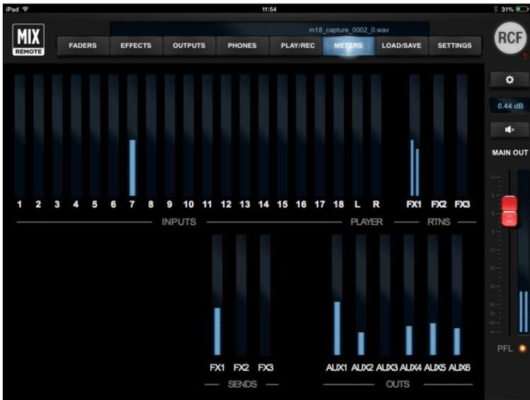
This tab has just page, which provides an instant view of the levels of all INPUTS - including the PLAYER - and of three FX stereo returns (RTNS).
