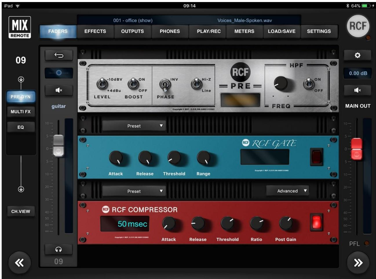
The -10dBV and +4dBu options are similar to the other line-level inputs; the **Boost** option allows you to insert another 2 dB boost to the analog stage; while the **Hi-Z** option enables a real high-impedance stage to get the best sound from your passive instrument. When in Hi-Z mode, the impedance is 1 M $\Omega$ . When using active instruments, we suggest maintaining the Hi-Z option OFF.
