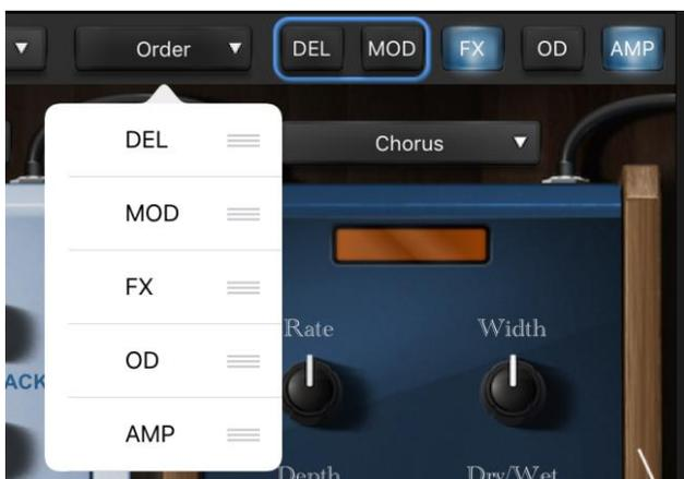
Similarly to channels 5 to 8, the effects are displayed in pairs, and you can jump to the desired insert effect by touching the dedicated button on top right (see the red box here below). You change effect daisy-chaining using the **Order** Selector, immediately to the left of the insert sequence indication. If you drag the rightmost part of the list, you can modify the insert position of a specific effect, and the change is effective immediately.
