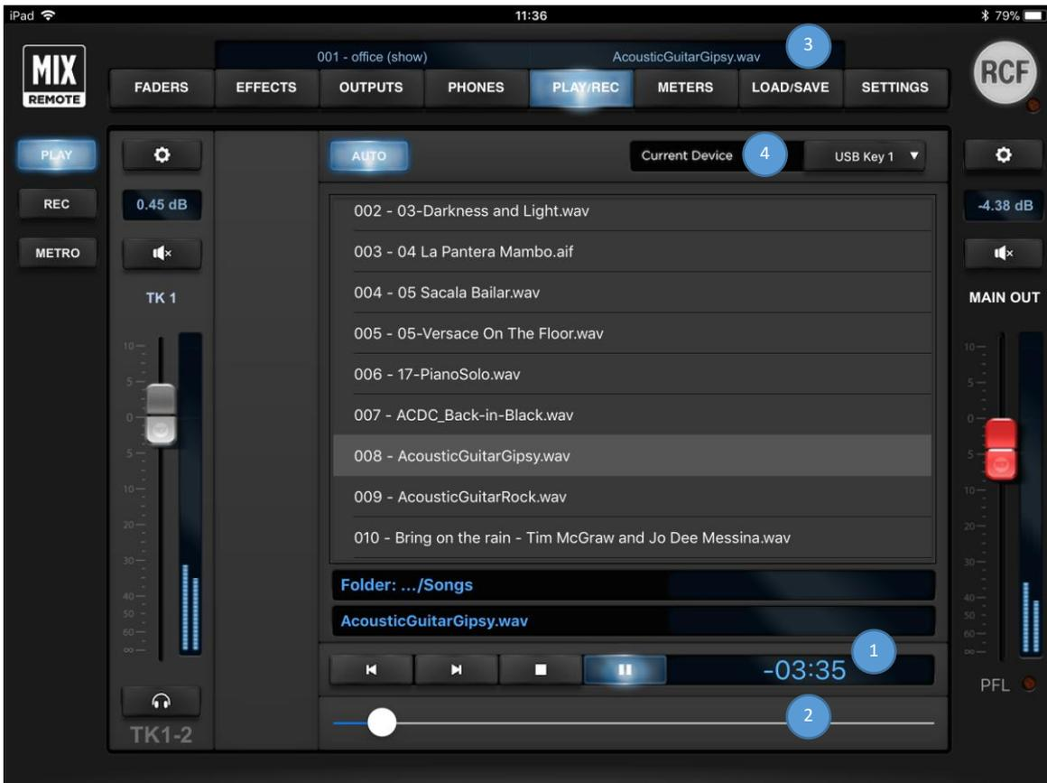
A large selection pane allows you to navigate through the USB flash drive folder (upper section), and then to select the specific files (lower section). To navigate to the previous directory, in the folder section, you can click on the line with 3 dots. *Please notice that with a very large amount of files, it takes several seconds to show all file names.*
