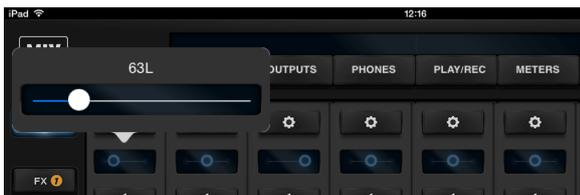
The central area is reserved for a view of 8 faders **(12)**; this area can be scrolled by swiping your finger horizontally. Above each fader there is a \* **(13)** to recall its setup pages, a box indicating the pan-pot position or each fader level in dB **(14)** and a Mute button **(15)**. Please note that clicking on the pan-pot, a larger windows opens, allowing better setting accuracy.
