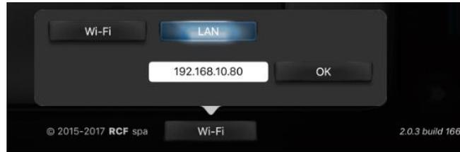
8. If connection fails, it may be due to the fact that the selected IP address is already assigned to another device; in this case, repeat from step 3 and type a different static address.
