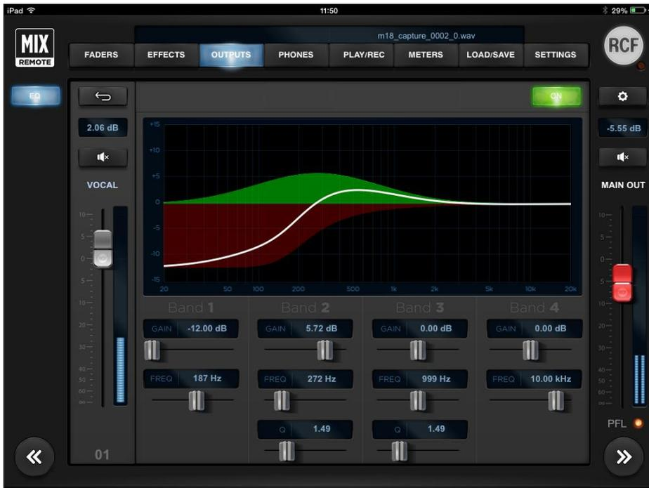
Pressing \*, you recall the OUTPUTS EQ page, containing the Advanced EQ for that AUX send; the other controls are for level and mute.
