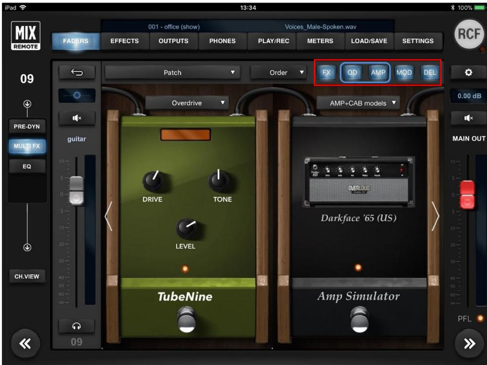
At the top of each pedal there is a display showing the last edited control value. At the bottom there is an activation switch; its status is displayed by a light, which is lit when the unit is on. The **OD** section allows choosing between an Overdrive and a Distortion effect, modeled after well-known stomp boxes that have been used by guitar players for decades.
