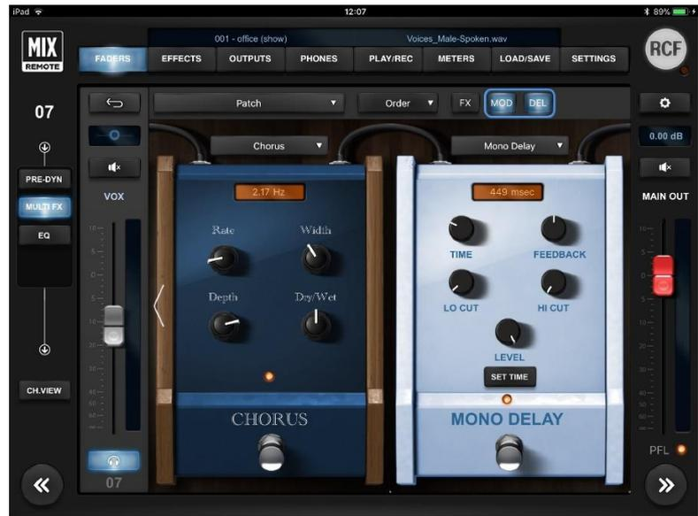
At the top of each pedal there's a display showing the last modified control value. At the bottom there's the activation switch; its status is displayed by a light which is lit when the unit is on.
