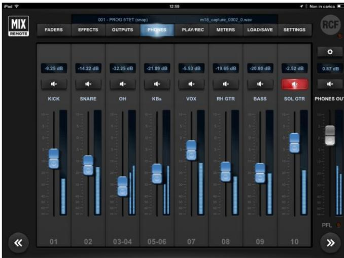
In **Personal Mix** mode, the central column of the PHONES page includes a box indicating the level of the individual fader in dB or the pan-pot position, a small Mute button, a text box which by default is the number of the send, which can be renamed, and a blue fader for headphone level and the non-editable number of the hardware socket. The level is pre-fader.
