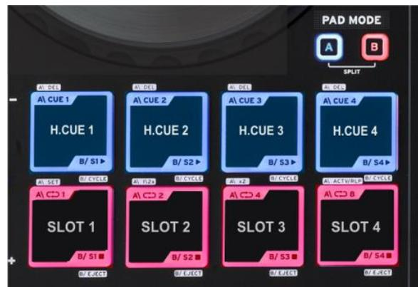
Hold **SHIFT** down and then press one of the 4 top pads to **delete** its assigned Hot Cue Point.
