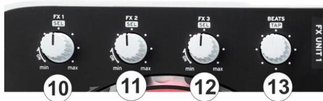
The Reloop Beatmix 2 offers 2 modes for the Effects control. In the **Multi Effect mode**, the effect units offer control for **3 Effect slots** with 1 effect parameter for each, while the **Single Effect mode** offers a **single Effect slot** but more effect parameters. Use the **SHIFT+PITCH-/+** (9/10) buttons to choose one or the other mode.
