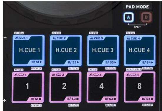
Hold **SHIFT** down and then press one of the 4 top pads to **delete** its assigned Hot Cue Point.
