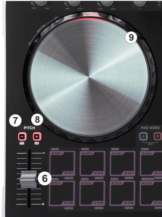
9. **JOGWHEEL.** Touch sensitive platter for scratching (vinyl mode), bending (CD Mode) or Seek mode. Touch the use the jogwheel to scratch and the outer ring to bend. Hold **SHIFT** down and then use the jogwheel to navigate through the track (seek mode)
