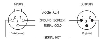
Mono input channel's mic input, Stereo input channel's mic inputs, Master section: T/B mic. Master section: Mix L, Mix R, Mix Mono, Grp 1-4 Aux 1-4, Matrix 1-2.
