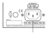
4 Connect AC mains power. Check first that the correct mains lead with sealed plug suitable for your local supply has been provided with your console. Plug into the AC MAINS IN socket making sure the connector is pressed fully in.
