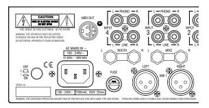
Read the **SAFETY INSTRUCTIONS** printed at the front of this User Guide and on the rear panel. Check that the correct mains lead with moulded plug has been supplied with your console. The power supply accepts mains voltages within the range 100-240V without changing any fuses or settings.
