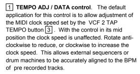
An internal jumper can be reassigned to change the function of this control to a dedicated DATA send, and will output Control Change CC94. See Service Options for details.
