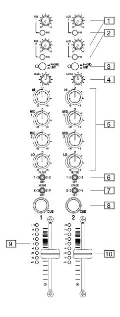
1 AUX 1-2 sends. Adjust the levels of the channel signals to the stereo Aux outputs. Turn fully anticlockwise to turn the signal off, fully clockwise for a maximum +6dB boost.
