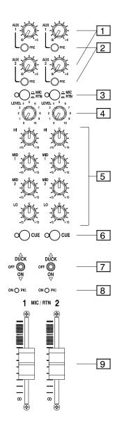
1 AUX 1-2 sends. Adjust the levels of the channel signals to the stereo Aux outputs. Turn fully anticlockwise to turn the signal off, fully clockwise for a maximum +6dB boost.
