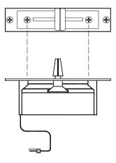
Use a medium size cross-point (Pozidriv) screwdriver to undo and remove the two outer screws on the crossfader plate. Do not remove the inner screws. Lift the crossfader assembly up and away from the console panel. Unplug the cable from the old crossfader and plug in the new assembly. Check that the connector is correctly aligned and pushed on. Replace the assembly making sure the cable faces the left side of the console. Refit the screws and test operation.
