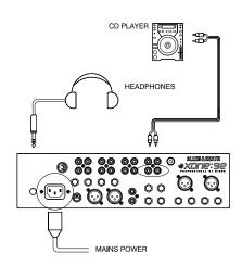
1 Set all controls to their starting condition. Set all FADERS (rotary and linear), LEVEL, AUX, FREQ, RESONANCE, LFO DEPTH, HEADPHONES and BOOTH MONITOR controls to minimum. Set EQ controls to their detented centre position. Set all press switches to their up position. Set all toggle switches to their centre position.
