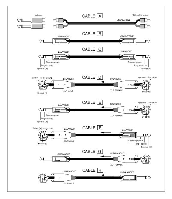
The CH1-2 MIC input. Balanced XLR. Plug in a DJ, guest or announcement microphone here. Use good quality low impedance dynamic mics such as those specifically designed for vocals. Do not use high impedance or unbalanced microphones, or condenser types which require phantom power. Use professional grade balanced cables wired as CABLE D. Use the best cable and connectors you can afford as these are typically subject to intense use and abuse in the club environment.
