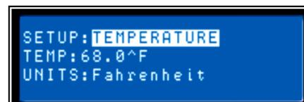
**Note:** Sound travels at different speeds depending on the density of the surrounding air it is traveling through. Cold air is denser than warm air thus, travels slower than it would if the air was warmer. Temperature can have a major influence with greater distances, particularly with respect to widely separated speaker arrays surrounding the audience for example. Temperatures might vary wildly between an indoor environment and an outdoor evening environment for example.
