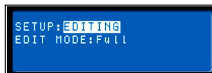
Regardless of the edit mode selected, there are two means to enter edit mode: pressing the Edit button or pressing any DSP block button.
