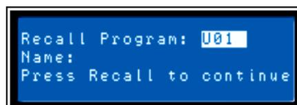
To recall a preset, press the front panel Recall button. The display switches to the Recall Preset screen and displays the next in a list of available presets in memory. Using the Value Up and Down buttons, select the preset to be recalled. Valid presets will display the preset name. Empty presets will display a “?”.
