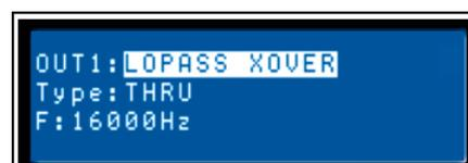
also be used to insure that low-frequency energy is not accidentally routed to the mid-range or tweeter drivers that may result in potential damage.
