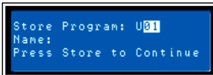
Press the < Select > buttons to navigate down to the preset name field. Use the Value Up and Down buttons to select the field for each letter / symbol character. The DSP 260 provides the complete ANSI character set, including lower-case & upper-case letters, numerals and symbols. Pressing and holding the Value Up and Down buttons will scroll rapidly through the character set. Press the < Select > buttons to move to the next or previous character position.
