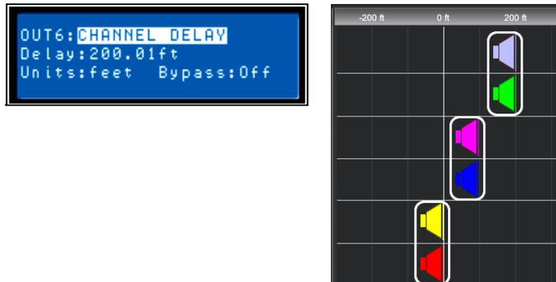
Illustration 5.3: Here Output 5 and 6 are linked and their delay is set to 200 feet. Output 3 and 4 are also linked and set to 100 feet. In this configuration, speaker outputs 5 and 6 are said to be 200 feet in front of Main speaker output array 1 and 2. The effect of air temperature on the actual delay time will also be automatically calculated based on the Temperature Parameter in the Setup Menu. See Output Linking.
