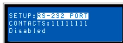
Contacts allow control messages to select individual presets (per pin 1-9) using a remote device. The additional CONTACTS parameter is used as a display only and corresponds to the binary values of individual pins, ie - on/off.
