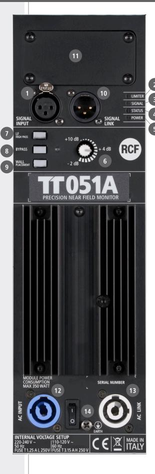
The XLR connectors use the following AES standard: PIN 1 = GROUND (SHIELD) PIN 2 = HOT (+) PIN 3 = COLD (-) HOT
