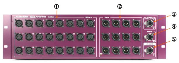
**D** Input sockets 24 balanced XLR inputs for microphone and line level sources. The preamps are built into the AR2412 rack and their Gain, Pad and 48V phantom power is remote controlled from the mixer via the dSNAKE link. The output of the analogue preamps are converted to digital format and transported via dSNAKE to be processed and mixed at the GLD or Qu mixer.
