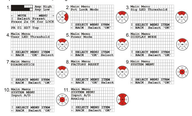
Press the marked arrow keys of the navigation-pad one after another (like shown in the scheme), to switch the input of channel A to "analogue" / "digital L" resp. "digital R" or "digital L+R" (the selection can be looked up from the LCD display from the respective direction of arrow). After the correct selection of the input press the OK-button and leave the menu with the left arrow key.
