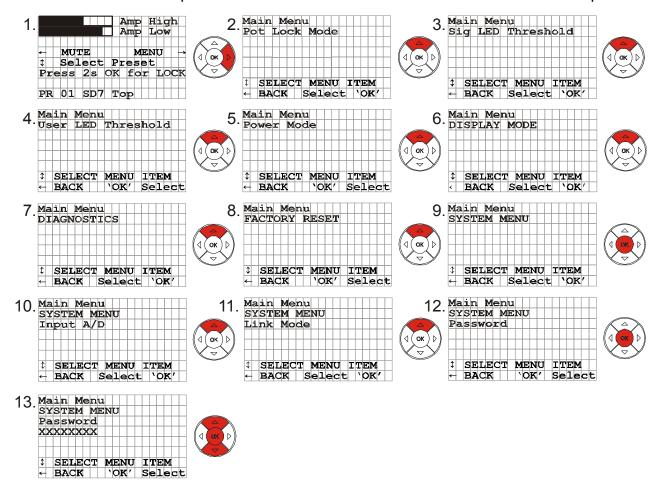
Press the marked arrow keys of the navigation pad one after another (like shown in the scheme) to open the sub menu "password". Now you can enter your password with the arrow keys and confirm with OK. You can leave the menu by pressing the left arrow key.
