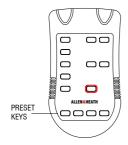
**Working with presets** The optional **PL-5** infra-red hand-held controller adds the presets function. Up to 4 level and source selection combinations may be stored in the **PL-12** memory. This is convenient for quick recall of settings for regular events. The installer can store these during installation, then use menu option 7 to disable store to prevent them being overwritten by the operator. To disable preset recall use menu option 6.
