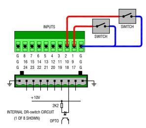
**Using the switch closure inputs** The input is opto-coupled to isolate the **iDR-switch** from the connected equipment. It is switched by linking its connector pin to the ground ('G') pin. Use a contact closure such as a momentary press switch to do this.
