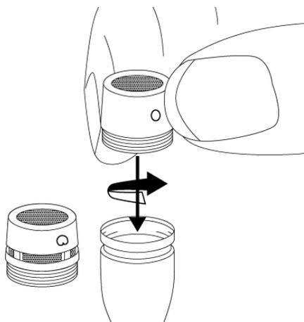
Microflex microphones use interchangeable cartridges that allow you to choose the polar pattern for different installations.
