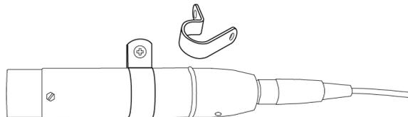
Use the two supplied mounting clamps to hold the preamp in place on a wall or ceiling.
